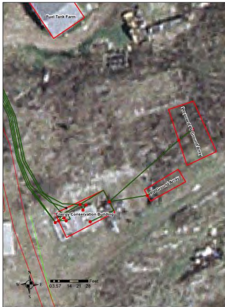
Figure 4: Energy Conservation Building (ECB) schematic of the new green grid. Note that the green lines and red points represent the new green grids electric lines and components, respectively.
