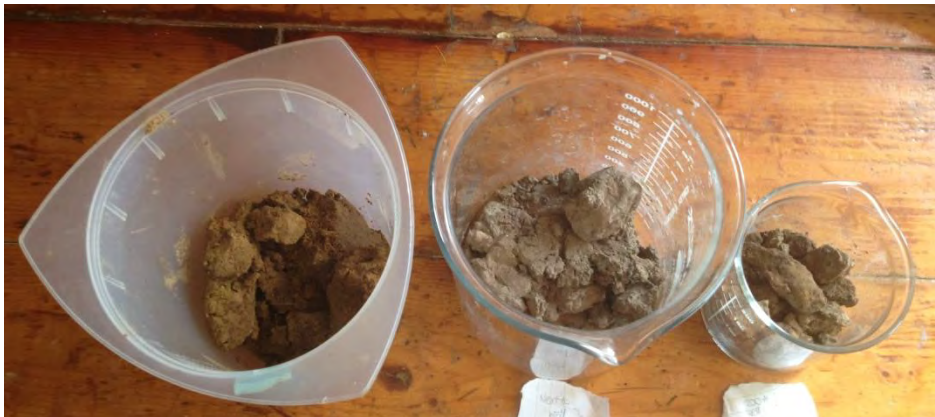
Figure 13: Samples from left to right: 100 feet, 2 feet, and 200 feet from the 20-foot dug well.
