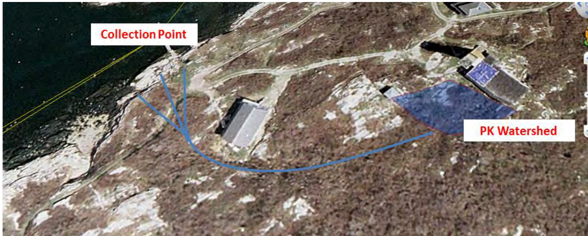
Figure 11: Aerial view of projected stream run-off from the PK watershed to the run-off collection point near the high-tide dock. The change in elevation is from 57 feet at the PK watershed to about 20 feet at the collection point.
