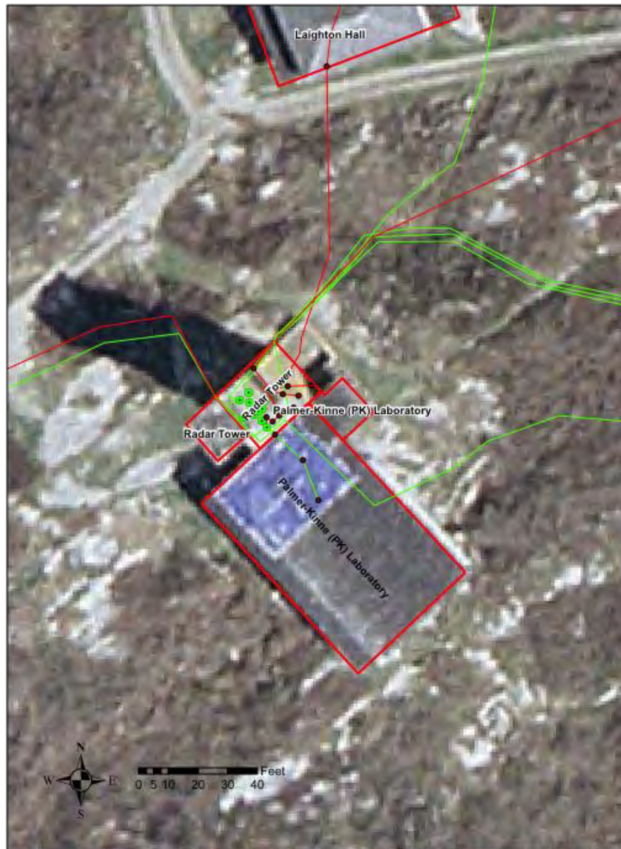
Figure 3: Radar Tower schematic of existing green grid. Note that the green lines and points represent the existing green grid electrical lines and electrical equipment, respectively. The red lines and points represent the dirty grid electrical lines and equipment.
