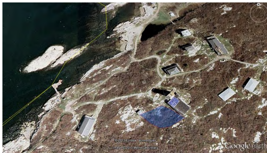
Figure 9: Aerial view of the proposed well watershed watershed by the Palmer-Kinne Lab. The elevation gradient of the watershed is about 0.092 ranging from 64 feet above sea level to about 56. The approximate watershed area is 9757.08 ft 2 .
