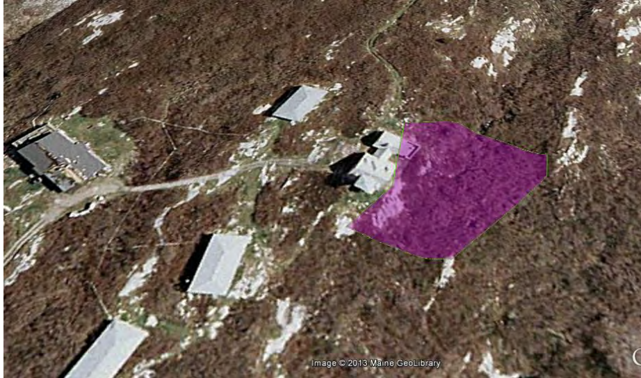
Figure 10: Aerial view of the proposed well watershed behind Bartels. The elevation gradient of the watershed is about 0.124 ranging from 66 feet above sea level to about 53. The approximate watershed area is 9756.08 ft 2 .
