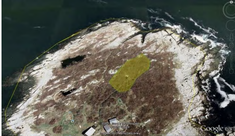
Figure 8: Aerial view of the 20-foot dug well watershed on the northern part of the island. The greatest elevation gradient of the watershed is about 0.119 ranging from 36 feet above sea level to about 26. The total approximate area was calculated to be 61603.26 ft 2 .
