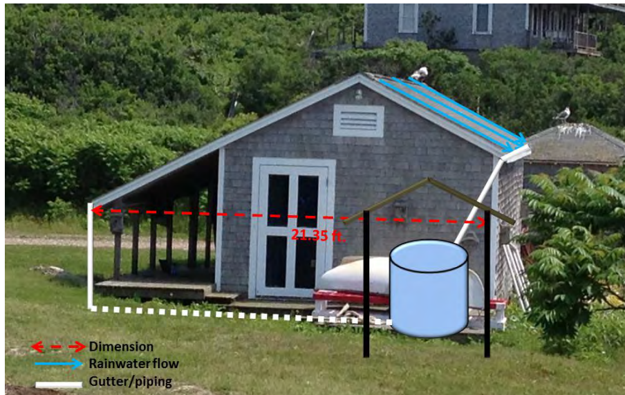
Figure 6: Side view of the Dive Shack, with a vertical 550 gallon HDPE cistern for catchment and a covering to protect it from the elements.
