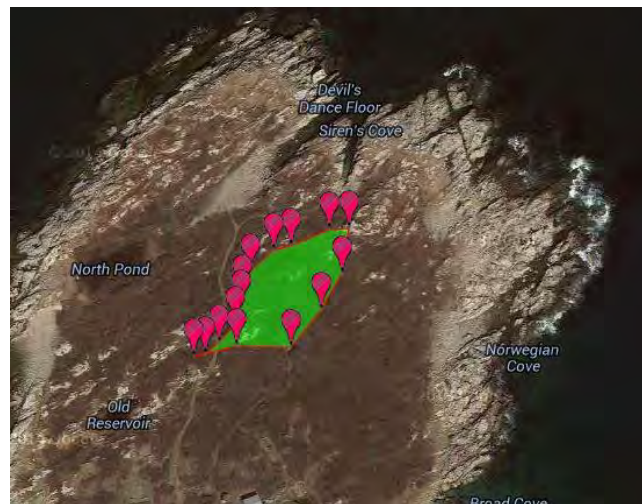
Figure 6.1: Watershed calculation on software program Daft Logic. The area was first found on Google Earth and the surface area calculated by using the pink markers as borders.
