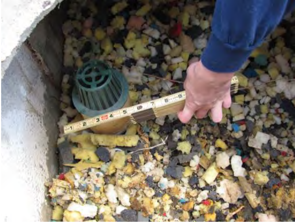
Figure 7.4 - Foam media in section 3 shows no sign of anaerobic activity, and still retains its natural color.
