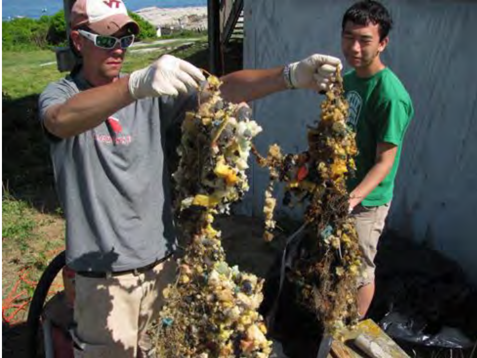
Figure 7.5 - Root system attached to foam media in FRICKle Filter™
