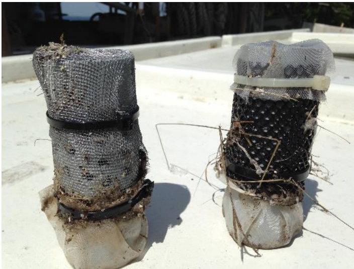
Figure 70: Filter A (left) and Filter B (right)
