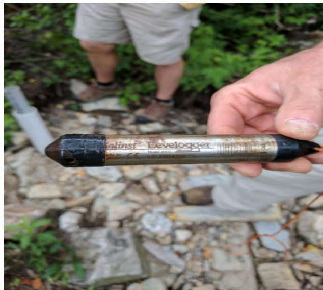
Figure 30. Levelogger that was used to read water level data in each of the wells
