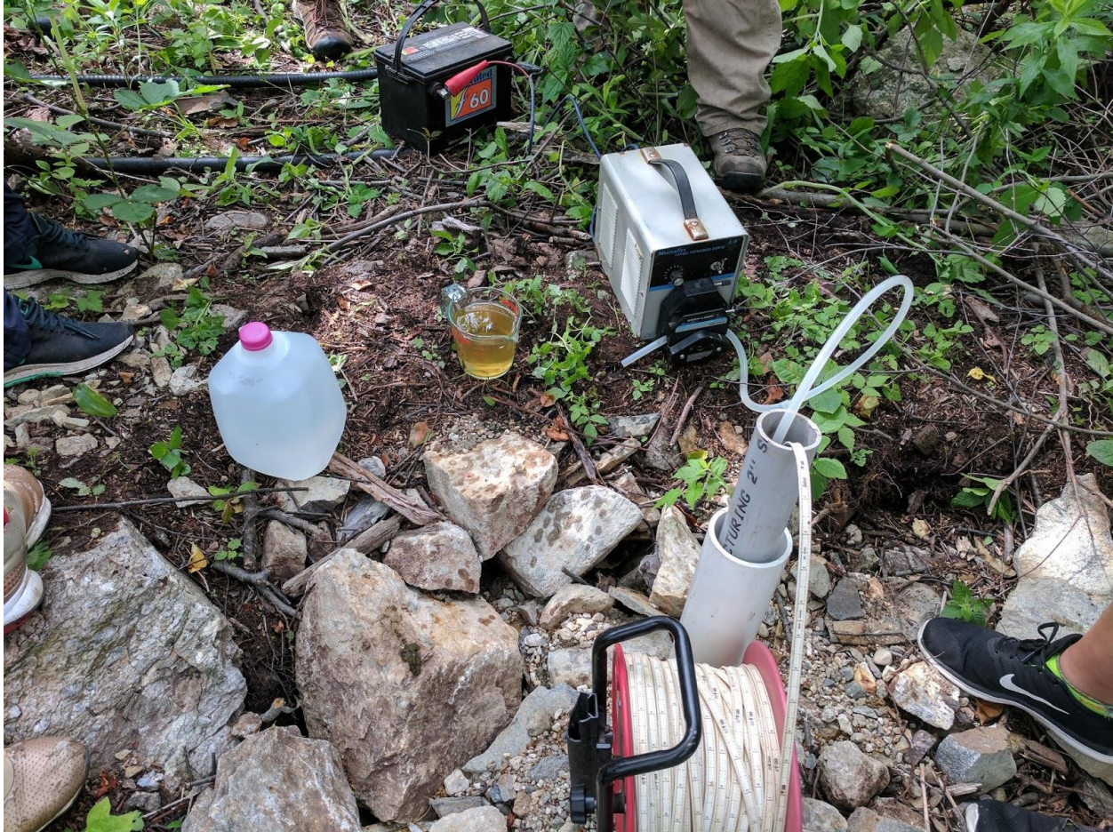
Figure 31. Set-up for the slug and pump tests at the six-foot well
