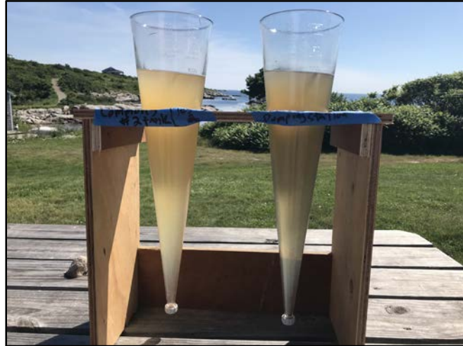
Figure 31: Imhoff Cone Samples Taken from Distribution box (Dorms- left , Main- right )
