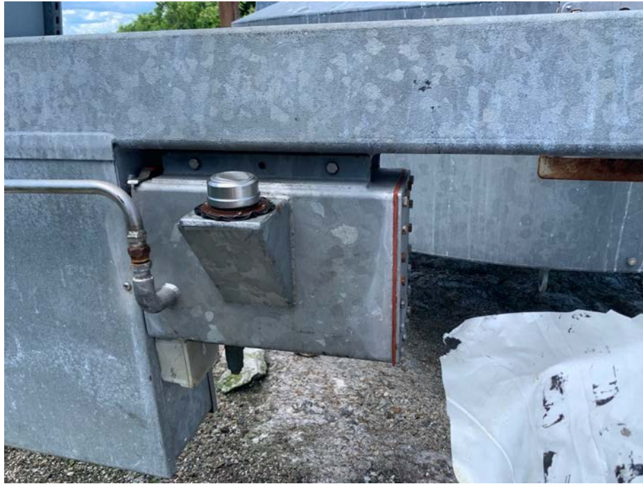
Figure 1.3: Hydraulic reservoir tank. The right side is a separate sheet of metal bolted to the rest of the tank and fitted with a gasket.
